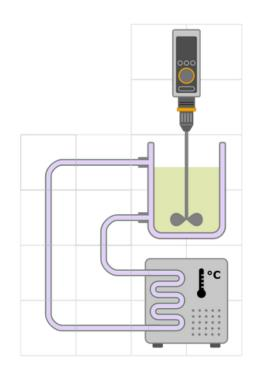
**Start simple** - This basic version includes an overhead stirrer and a thermostat and enables you to program the basic environmental parameters for chemical reactions. The stirrer speed can also be controlled by the temperature in the vessel.
