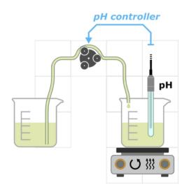
This device combination allows you to reach and control the desired pH in your vessel: when the measured pH is below your target, an alkaline solution is pumped into your vessel.
