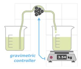
With this device combination, you can dose solutions reliably, accurately, and automatically. You set in the software UI the mass of solution you want to add to your vessel and the pump dispenses it automatically based on the feedback from the scale: when the target amount is reached, the pump stops.
